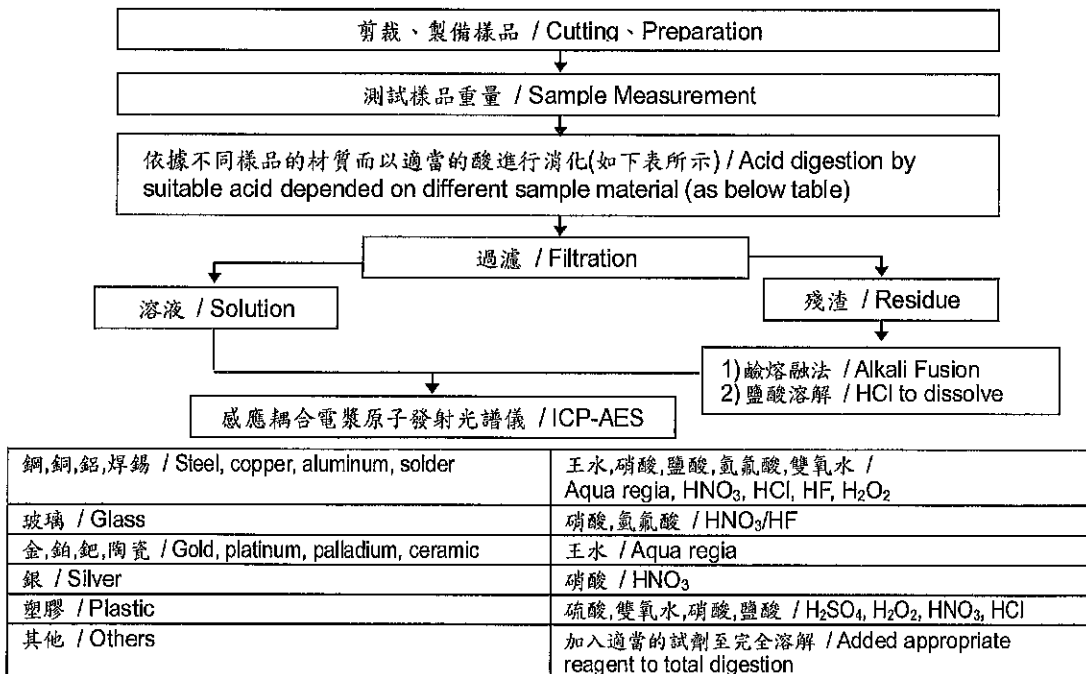
元素以 ICP-AES 分析的消化流程圖 (Flow Chart of digestion for the elements analysis performed by ICP-AES)
