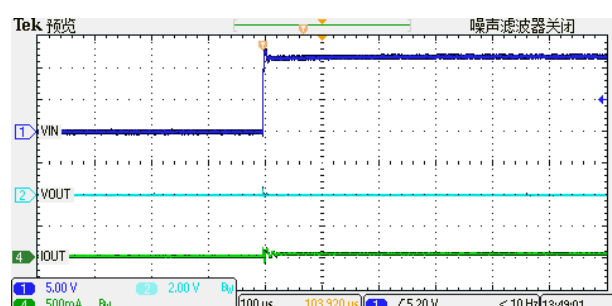
Short circuit on Power V_{OUT}=12V, 100\mu s
