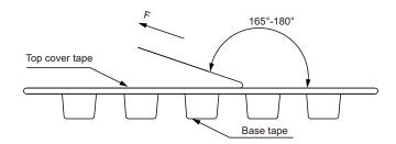
The peel force of top cover tape shall be between 0.10 to 1.17  $\mbox{N}$
