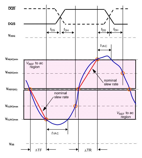
Setup Slew Rate Falling Signal =
