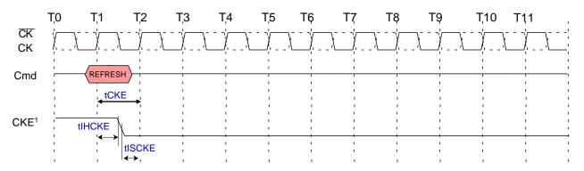
NOTE 1 CKE can go LOW tIHCKE after the clock on which the REFRESH command is registered.
