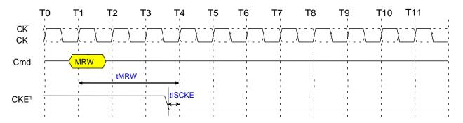
NOTE 1 CKE can be registered LOW tMRW after the clock on which the MRW command is registered.
