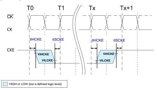
NOTE 1 After CKE is registered LOW, CKE signal level shall be maintained below VILCKE for tCKE specification (LOW pulse width).
