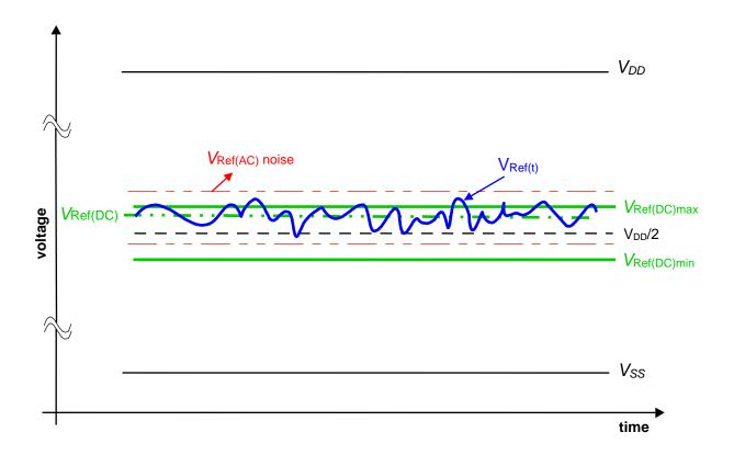
The voltage levels for setup and hold time measurements  $V_{IH(AC)}$ ,  $V_{IH(DC)}$ ,  $V_{IL(AC)}$  and  $V_{IL(DC)}$  are dependent on  $V_{Ref}$ . " $V_{Ref}$  " shall be understood as  $V_{REF(DC)}$  above.
