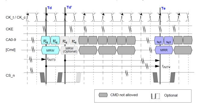
NOTE 1 Optional MRW RESET command and optional  $\overline{\text{CS}}$  assertion are allowed, When optional MRW RESET command is used, tINIT4 starts at Td'.
