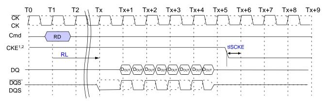
NOTE 1 CKE must be held HIGH until the end of the burst operation.
