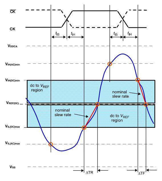
$$\begin{array}{c} \text{Hold Slew Rate} \\ \text{Rising Signal} = \frac{V_{\text{REF(dc)}} - V_{\text{IL(dc)}} \text{max}}{\Delta \text{TR}} & \text{Hold Slew Rate} \\ \text{Falling Signal} = \frac{V_{\text{IH(dc)}} \text{min} - V_{\text{REF(dc)}}}{\Delta \text{TF}} \end{array}$$
