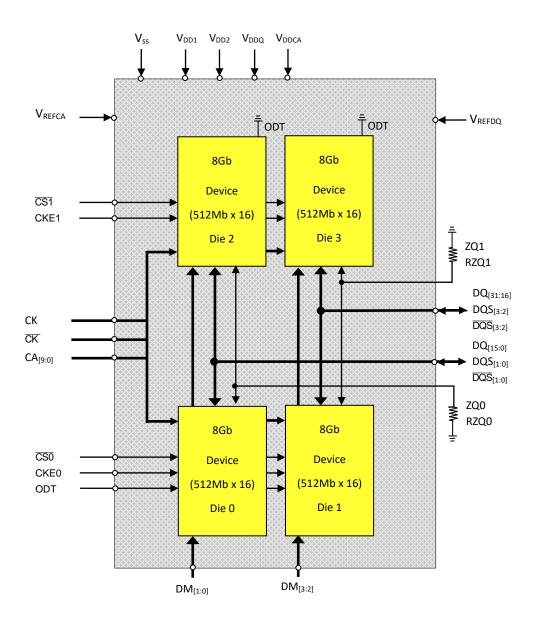
NOTE 1 ODT will be connected to rank0 (die0/1). The ODT input to rank1 (die2/3) will be connected to VSS in the package.
