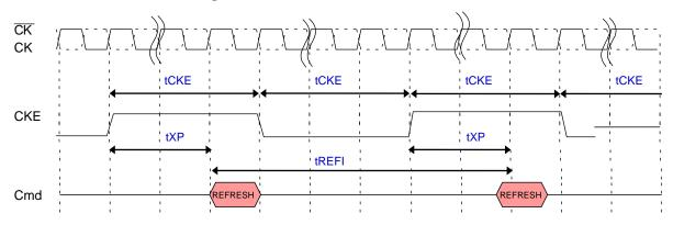
NOTE 1 The pattern shown can repeat over an extended period of time. With this pattern, all AC and DC timing and voltage specifications with temperature and voltage drift are ensured.
