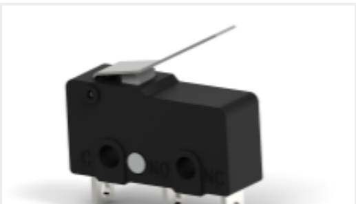
TE Part #2351456-1 SMINSA SW 18UPLV 1.47N 5A/3A AC 3A DC SP
