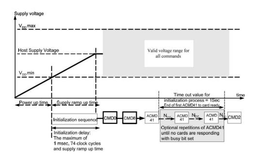
'Power up time' is defined as voltage rising time from 0 volt to VDD min.
