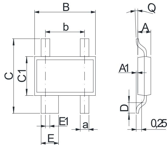
**Dimensions In Millimeters(SOT-143)**
