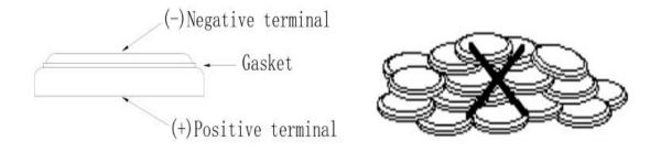
(2).The Batteries Put in a Metallic Container or on a Metallic Plate . (将电池放入金属容器或金属盘里)
