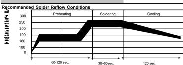
Recommended reflow methods: IR, vapor phase oven, hot air oven.
