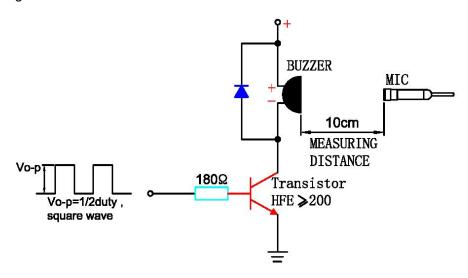
In the measuring test, buzzer is placed as follows:
