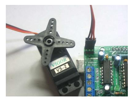
Hobby servos are the easiest way to get going with motor control. They have a 3-pin 0.1" female header connection with +5V, ground and signal inputs. The motor shield simply brings out the 16bit PWM output lines to two 3-pin headers so that its easy to plug in and go. They can take a lot of power so a 9V battery wont last more than a few minutes.
