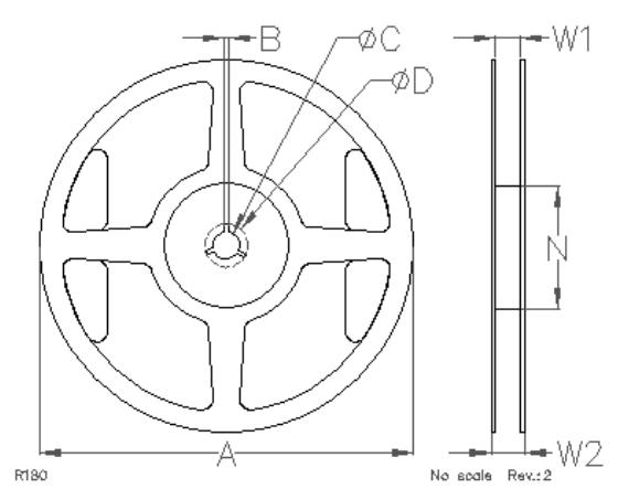
Note 1: All dimensions in [mm]. Dimension W1 is measured near the Hub (N).
