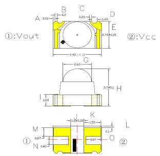
注/ Notes: 1. 单位:毫米 (mm) / All dimensions are in millimeters 公差: 如无特别标注则为± 0.1 mm Tolerance is ± 0.10 mm unless otherwise noted
