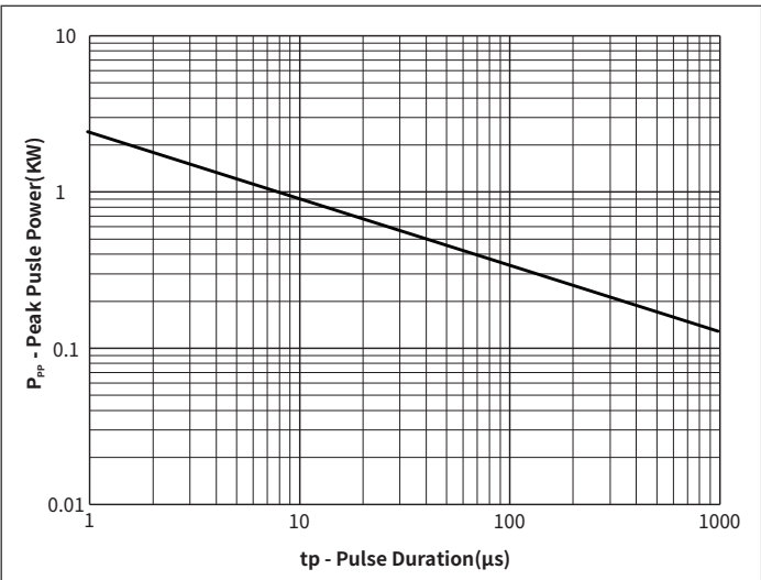
Fig.3 Peak Pulse Power vs. Pulse Time
