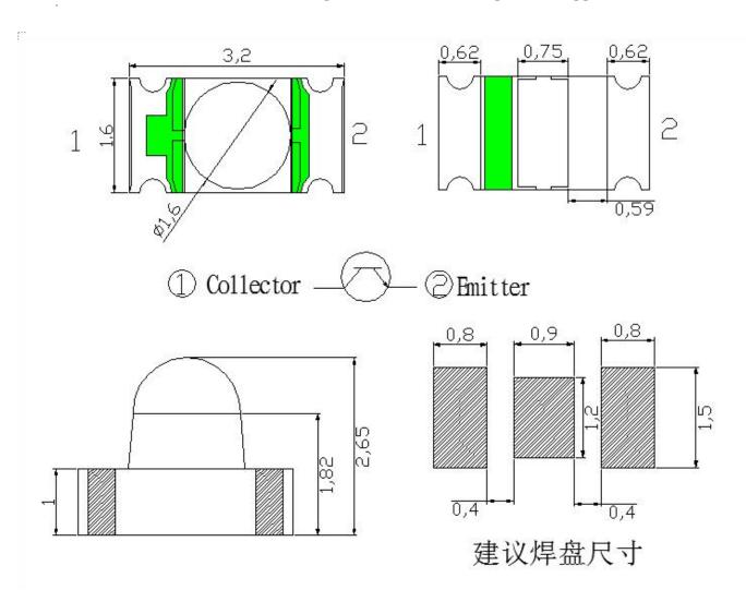
注/ Notes: 1. 单位:毫米 (mm) / All dimensions are in millimeters 公差: 如无特别标注则为± 0.1 mm Tolerance is ± 0.10 mm unless otherwise noted
