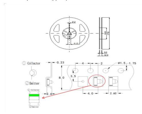
注/ Notes: 1. 尺寸单位为毫米(mm)/ All dimensions are in millimeters.
