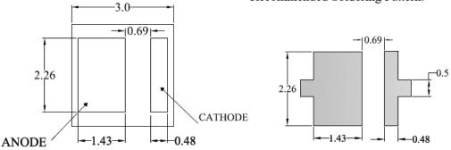
注/Notes: 1. 单位:毫米(mm)/All dimensions are in millimeters
