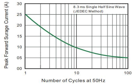
Fig.5 Maximum Non-Repetitive Peak Forward Surge Current
