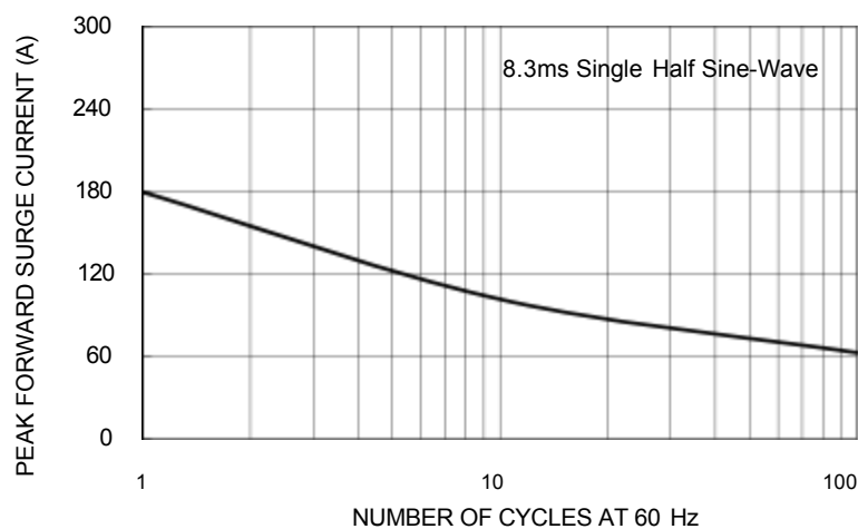
FIG. 3 MAXIMUM NON-REPETITIVE FORWARD SURGE CURRENT
