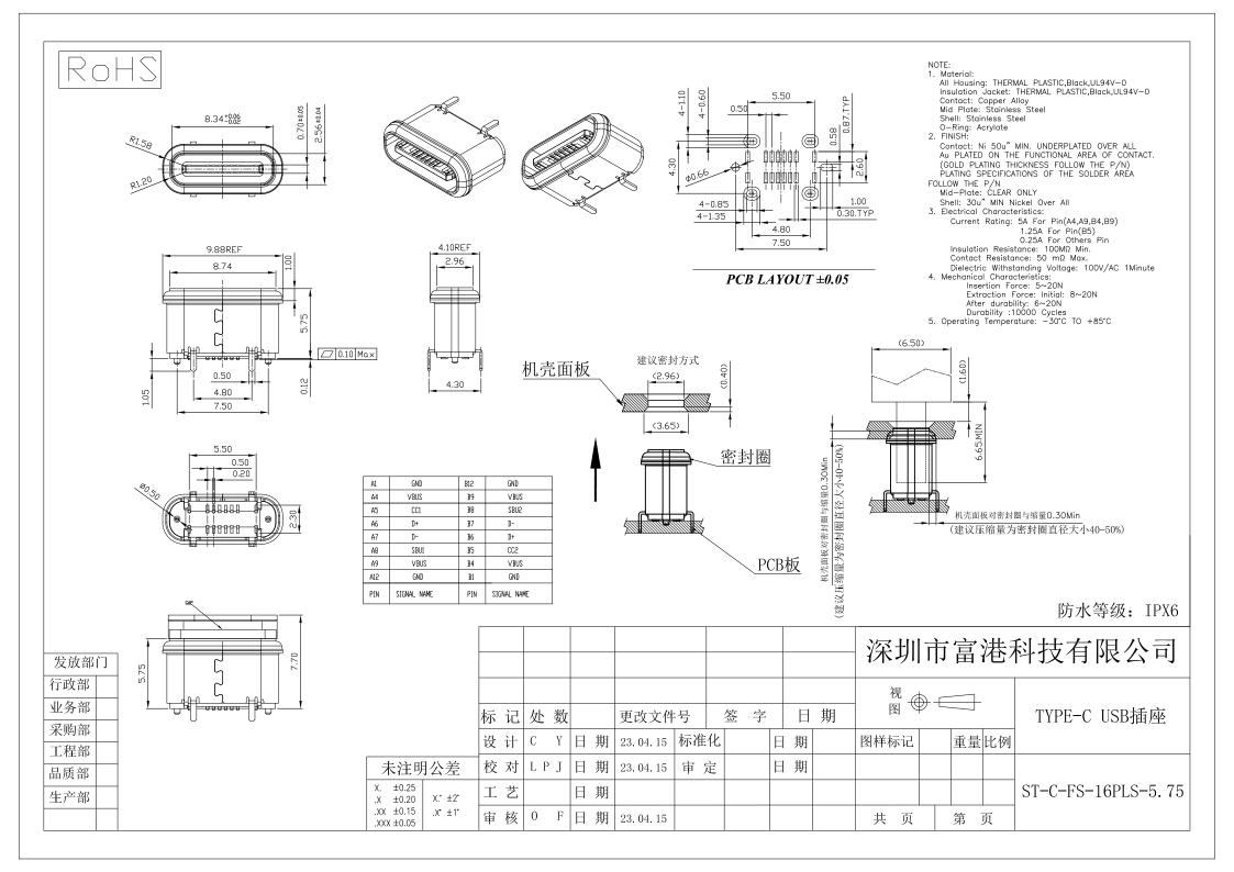
1.0 Scope: This specification covers the requirements for product performance and test methods of USB C TYPE Series Connectors of the part numbers specified as bellow.
