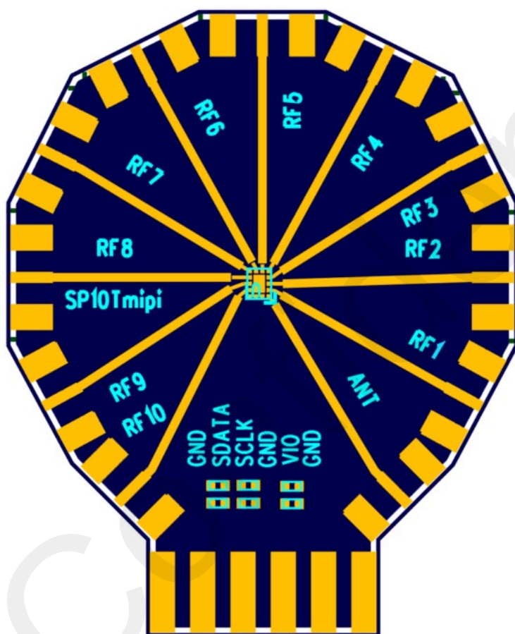
Figure 4 Evaluation Board Assembly Diagram
