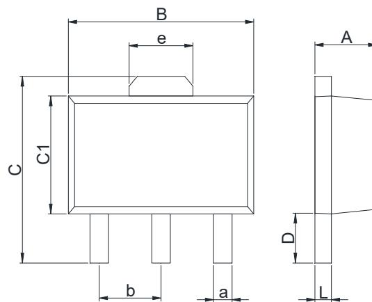
Dimensions In Millimeters(SOT-89-3)
