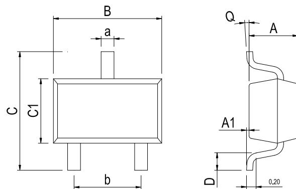
Dimensions In Millimeters(SOT-23-3)
