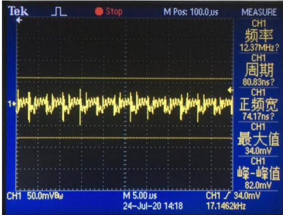
Ripple wave (VIN = 57V, IO = 2A, 5 ~ 20MHz bandwidth)
