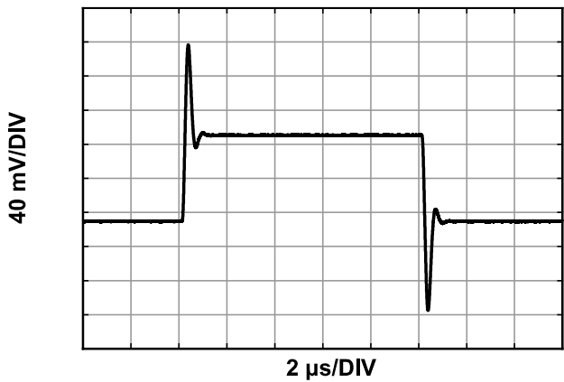
Figure 26. Small Signal Pulse Response ( G = 1 , R_L = 2\text{ k}\Omega , C_L = 100\text{ pF} )
