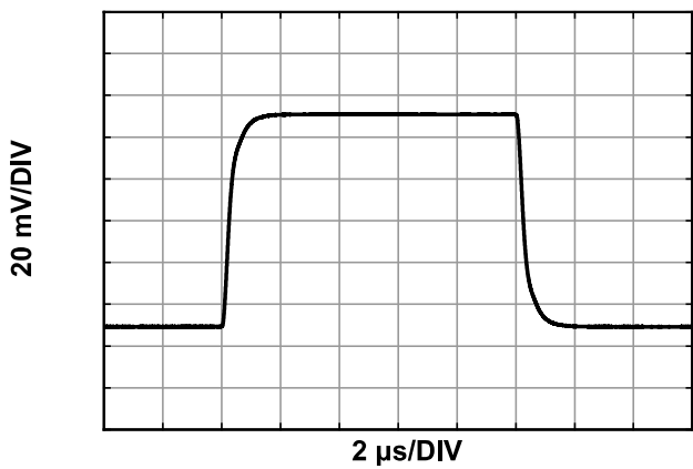
Figure 27. Small Signal Pulse Response ( G = 10 , R_L = 2\text{ k}\Omega , C_L = 100\text{ pF} )
