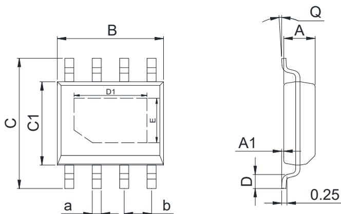
Dimensions In Millimeters(ESOP-8)
