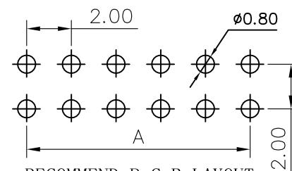
PCB TOLERANCE: ±0.05 (TOP VIEW)
