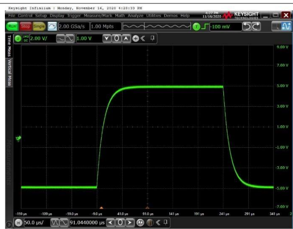
Voltage: 2V/div for Output, Time: 50us/div G=1000, VREF = GND; VIN=10mVPP, Load R=10K C=100pF
