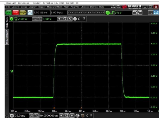
Voltage: 2V/div for Output, Time: 20us/div G=100, VREF = GND; VIN=0.1VPP, Load R=10K C=100pF
