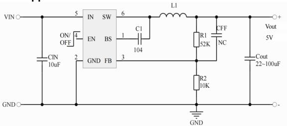
NOTE: Chip MLCC capacitors are recommended for typical circuits.
