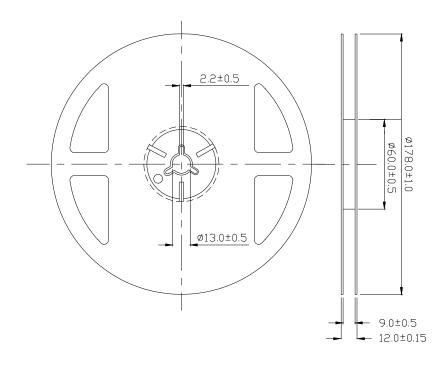
**Note:** The tolerances unless mentioned is  $\pm 0.1$ mm ,Unit = mm Carrier Tape Dimensions :( Quantity: 1500pcs/reel)
