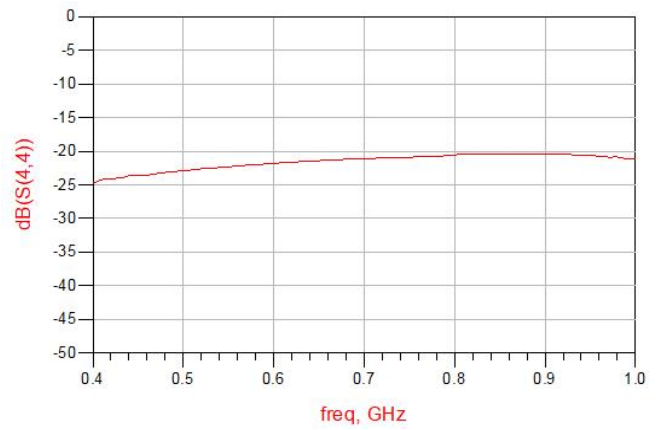
Figure 8. MHC0410L03 Return Loss (S44)
