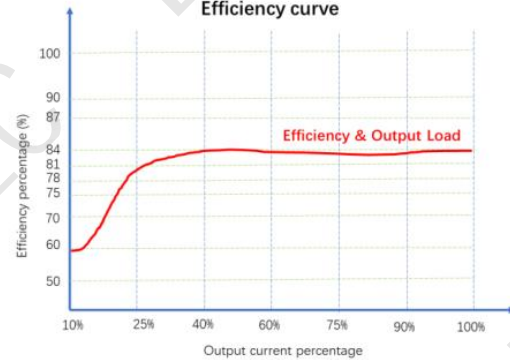
Figure 5: Efficiency VS Output Load (Nominal Voltage Input)
