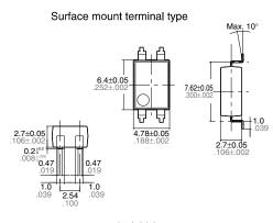
Terminal thickness: t = 0.2 General tolerance: ±0.1
