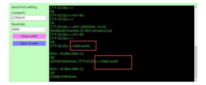
In user define mode, the user can input AT command to do the debugging
