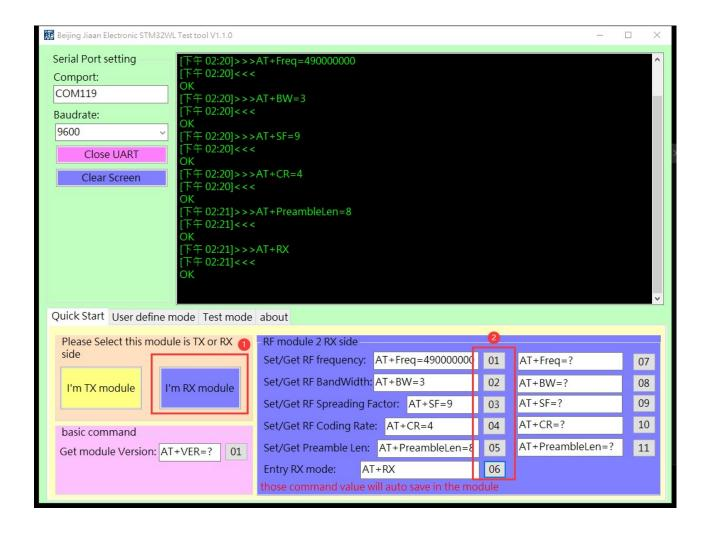
Then we prepare another module to be the transmitter and execute the following instructions in sequence. Finally, 06 will send out a string of Hello world. When sending out, if a module is in the receiving mode, it will receive data.
