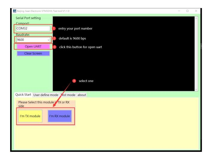
The following figure shows the setting page of Rx mode, and send all the 01-06 instructions in sequence once, that is to complete the module setting of Rx end. When the last instruction AT + Rx is executed, the mode will always be in the receiving mode.
