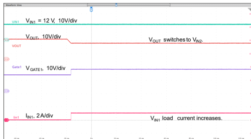
Figure 25. ORing: V_{IN2} Switches to V_{IN1}
