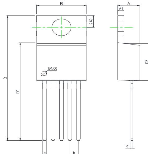
**Dimensions In Millimeters(TO-220-5)**
