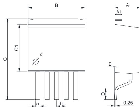
**Dimensions In Millimeters(TO-263-5)**
