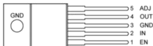
5-Pin TO-220 Adjustable Voltage LM29152/29302A/29502
