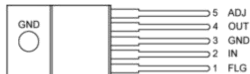
5-Pin TO-220 Adjustable with Flag LM29153/29303/29503
