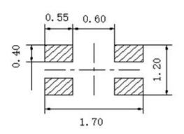
参考焊盘 Reference Soldering Pad
