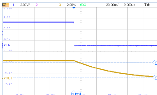
Turn Off Speed VS EN Voltage ( I_{OUT}=30mA )
