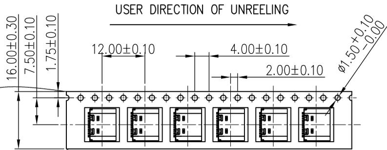
COVER TAPE PEELING ANGLE:  $165^\circ \sim 180^\circ$
