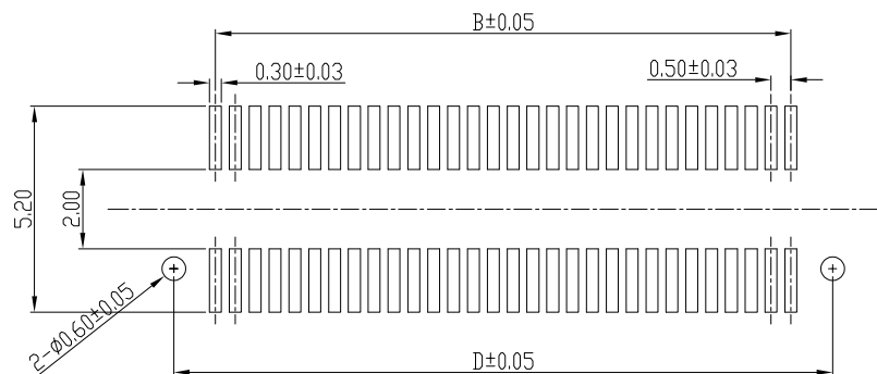
RECOMMENDED PCB LAYOUT(TOP VIEW)
