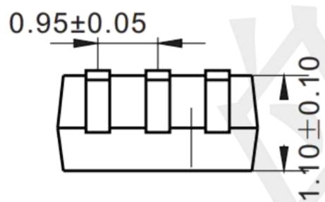
**Mounting Pad Layout (unit: mm)**
