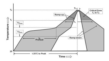
■ Recommended reflow methods: IR, vapor phase oven, hot air oven, N₂ environment for lead-free;
