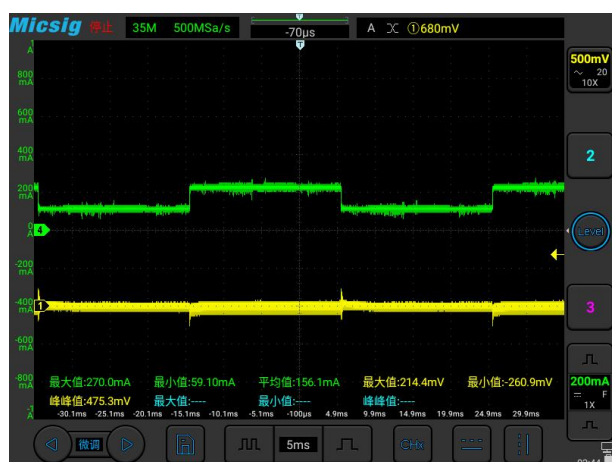
Transient Response VIN=52V, Io=50%~100%~50%
