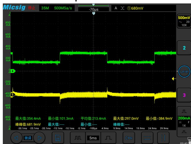
Transient Response VIN=52V, Io=50%~100%~50%
