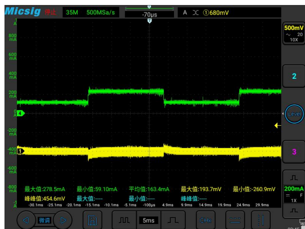
Transient Response VIN=52V, Io=50%~100%~50%
