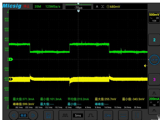
Transient Response VIN=52V, Io=50%~100%~50%
