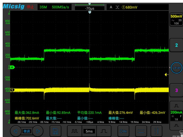
Transient Response VIN=52V, Io=50%~100%~50%
