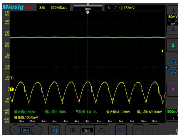
Noise V_{IN}=52V, I_o=1.8A 20MHz Bandwidth
