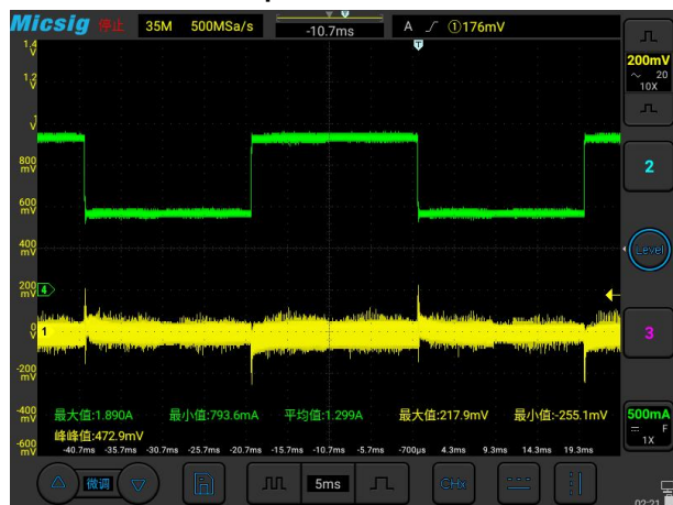
Transient Response V_{IN}=52V, I_o=50\% \sim 100\% \sim 50\%
