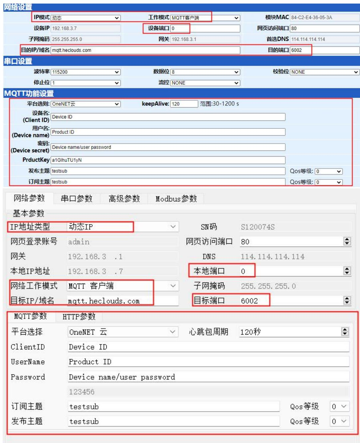
The screenshot shows the configuration interface for the NS1/NS1-TB module. The main sections are highlighted with red boxes:
