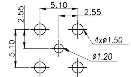
PCB.WELDING DRAWING (TOLERANCE:±0.05)
