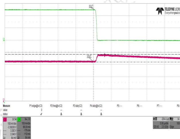
图 12. 负载响应 (250mA to 1mA IN 0.5us)
