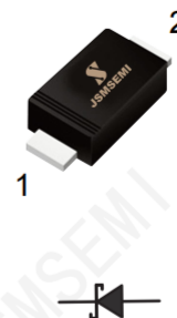
Top View Simplified outline SOD-123FL and symbol
