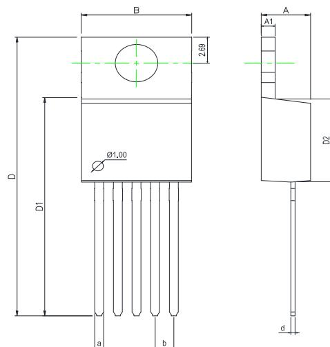
**Dimensions In Millimeters(TO-220-5)**
