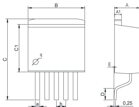
**Dimensions In Millimeters(TO-263-5)**
