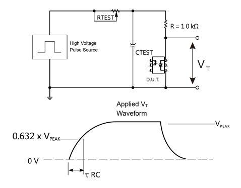
The high voltage pulse applied to the output end of the device under test through the RC circuit is set to the desired V<sub>PEAK</sub> value. LED current does not need to be added. Waveform VT is monitored with X100 probe. By adjusting the RTEST value, dv/dt (slope) increases until the device under testis observed to be triggered (waveform collapse). Dv/dt then drops until the device under test stops being triggered. At this time, dv/dt can be calculated by recording the value of TRC.
